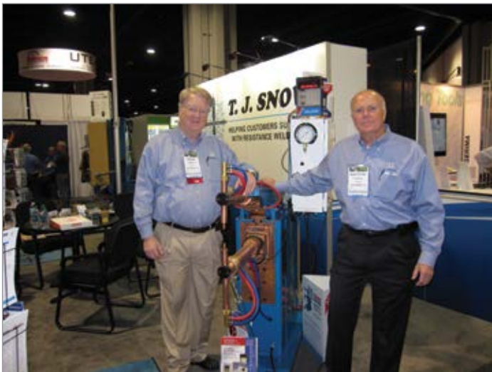
Thomas J. Snow and Mark Pepping (left to right) at the T.J. Snow booth with their new Rocker-Arm spot welding machine rated to consume five gallons per minute of chilled water.
