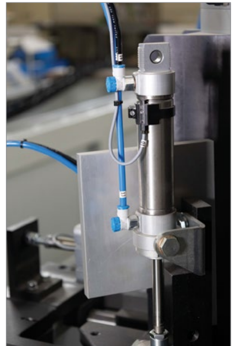
The diminutive Festo SDBT-MSX proximity switch, shown here affixed at the top of a round ISO cylinder, is the world's first such sensor with auto-teach-in, for simple, fast one-and-done commissioning.
