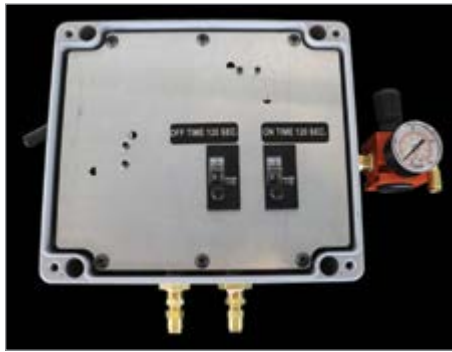
Pneumatic control components can be used to operate a compressed air dryer.
