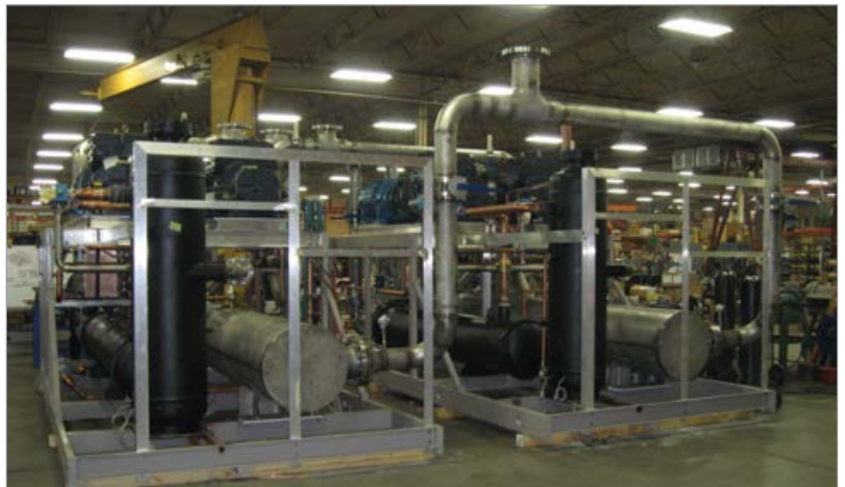
Low charge Ammonia is often the refrigerant of choice because it is safe, cost effective and energy efficient. The term low-charge indicates there is one pound or less per ton of refrigerant utilized.
