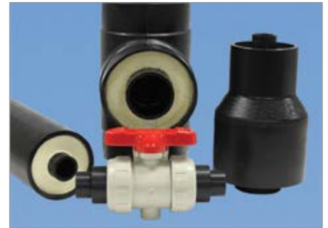
The new COOLSAFE™ provides thermal conductivity better than 0.026 W/m-K (0.015 Btu-ft/h-ft 2 -F).
