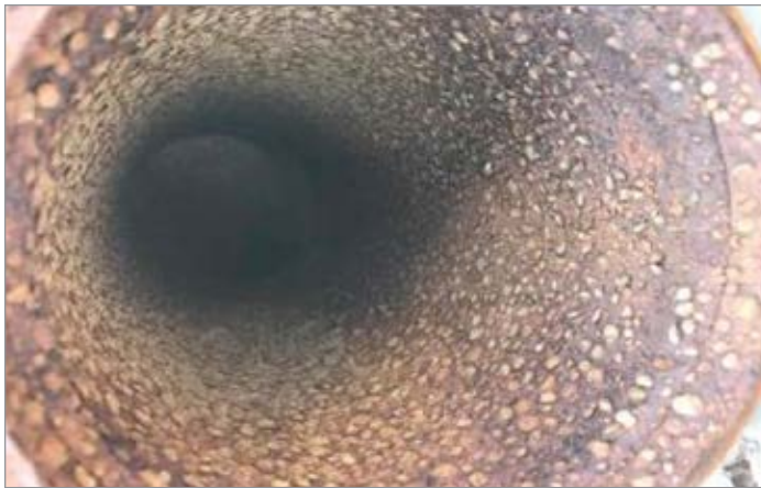
Cooling tower condenser tube exhibiting scaling and corrosion, before UET treatment.
