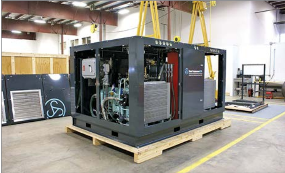
A high-pressure air compressor enclosure on the production floor.
