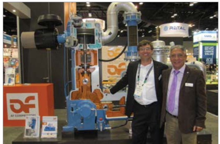
Joe Mashburn and Juan Manuel Ortiz, from AF Compressors, next to a cut-away of their 3-stage oil-free piston PET air compressor.
