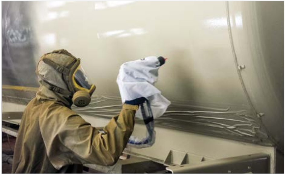
A high-efficiency electrostatic paint spray gun in operation
