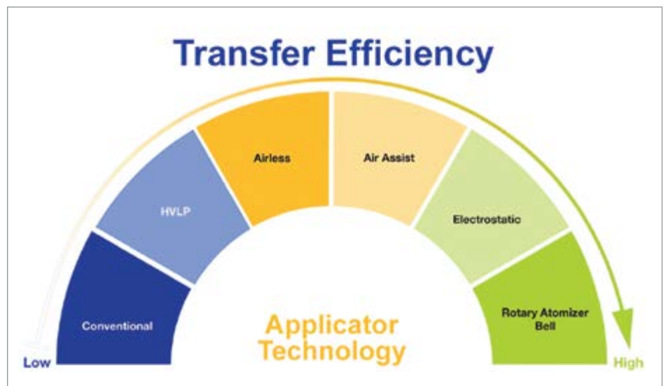
A comparison of different types of spray guns and their transfer efficiency (courtesy of Graco)
