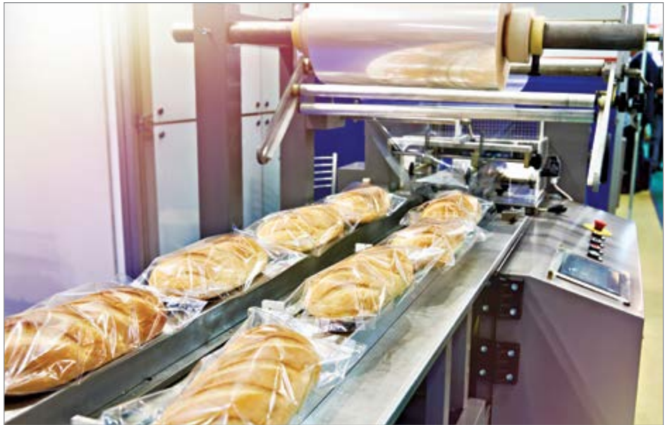
Direct-contact applications, where compressed air comes into contact with food products, may require a higher level of compressed air purity than indirect-contact applications such as running packaging machinery and conveyor systems.
