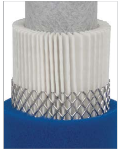
A coalescing inline filter removes both oil residue and fine particulates. With the right filtration, it is possible to meet food quality standards for compressed air with a lubricated air compressor.
