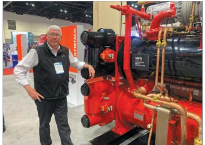
Pat Carus of Multistack with an MFH water-cooled MagLev® flooded heat recovery chiller.
