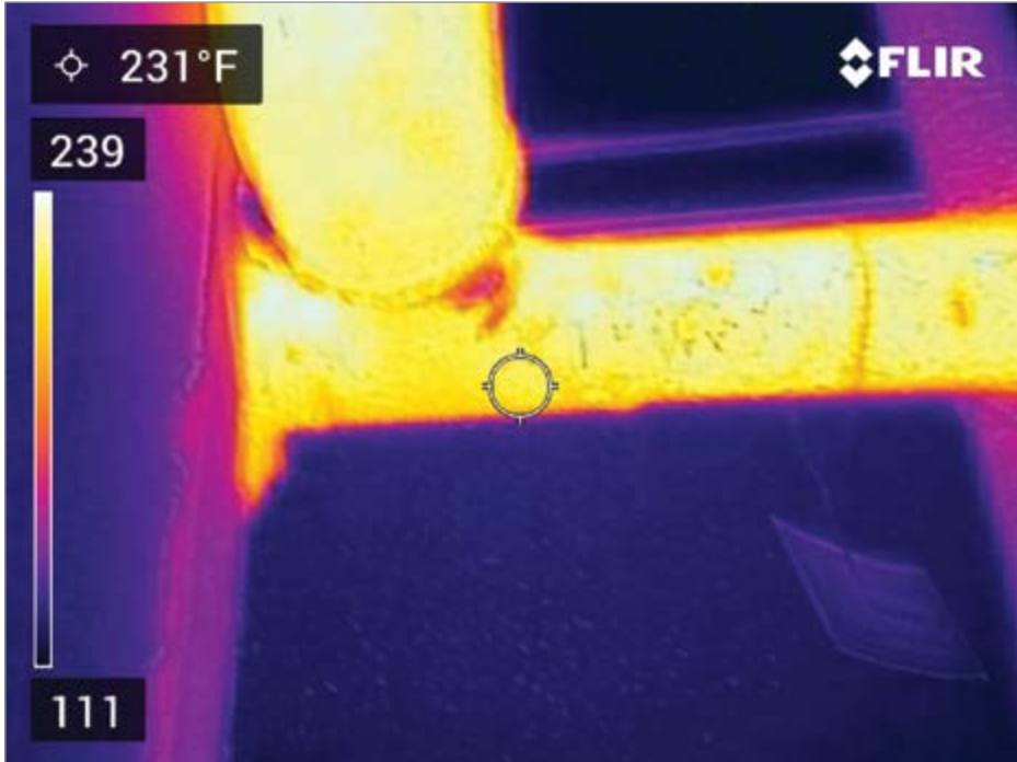
Neglecting insulation repairs, such as on this uninsulated steam line, can cost more than it saves.
