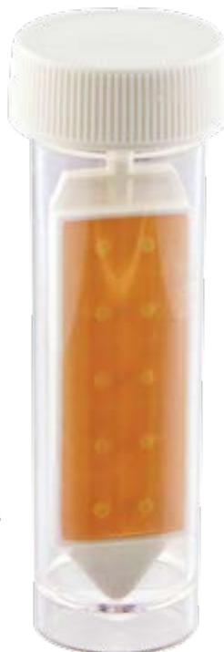
Figure 1. A Hach bacteria paddle tester
