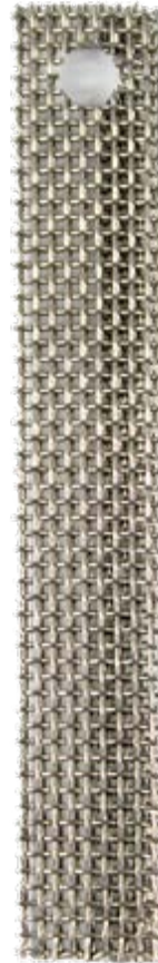
Figure 7. A stainless steel mesh test specimen from Pacific Sensor
