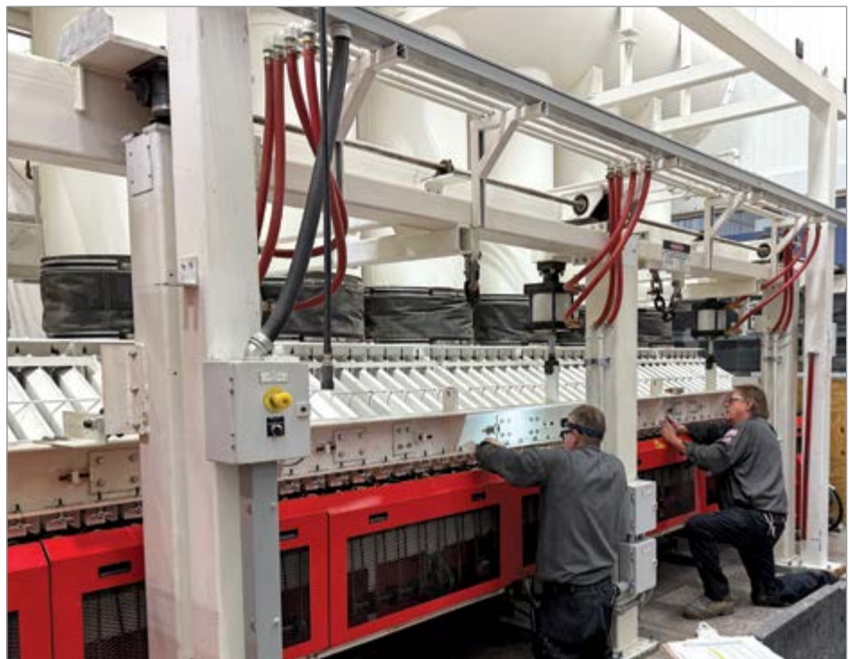
The quench system uses pressurized air to cool the glass.
