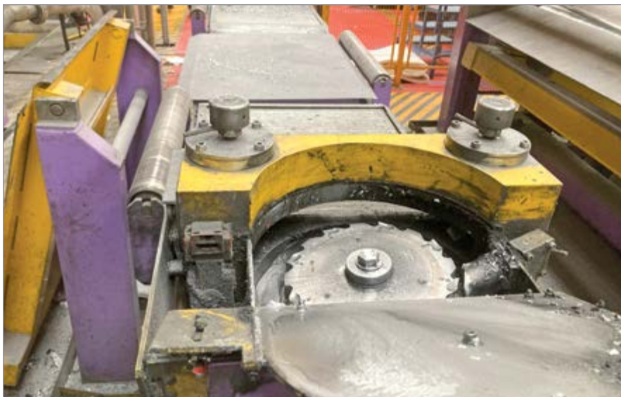
If the trimmed aluminum scraps aren't blown away, they'll get caught and wrapped into the foil during rolling.
