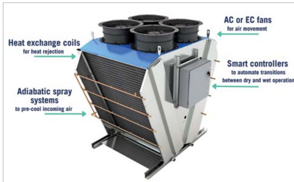
Image 3: Parts of an adiabatic spray cooling system
