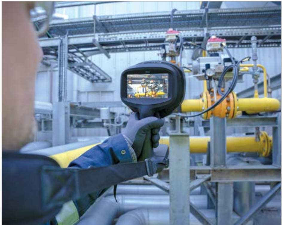
This acoustic imaging camera lets technicians detect and reduce compressed air leaks in industrial facilities, thereby cutting costs.
