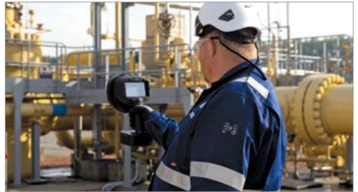
FLIR Si2x-Series enables reliable detection of pressurized gas leaks, mechanical faults and partial discharge in explosive vapor and dust environments.
