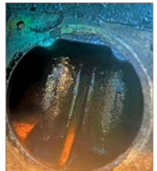
Varnish-coated surfaces reduce air compressor efficiency and component life, restricting cooling ability.
