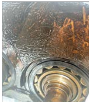
Varnish-coated surfaces reduce air compressor efficiency and component life, restricting cooling ability.
