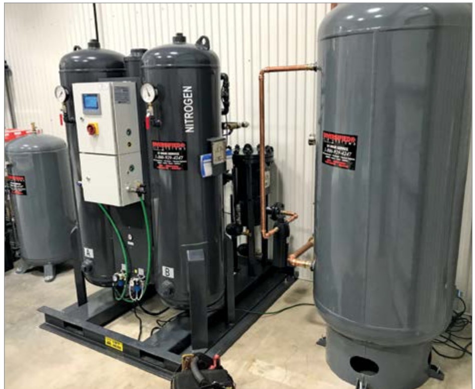
PSA nitrogen generators are the better choice when high-purity nitrogen gas is required.
