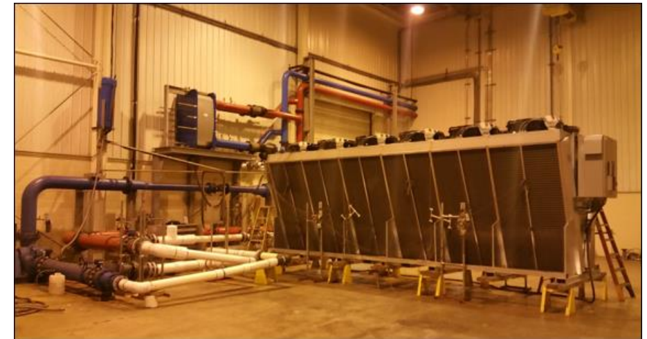
Dry cooler test in Evapco R&D Lab
